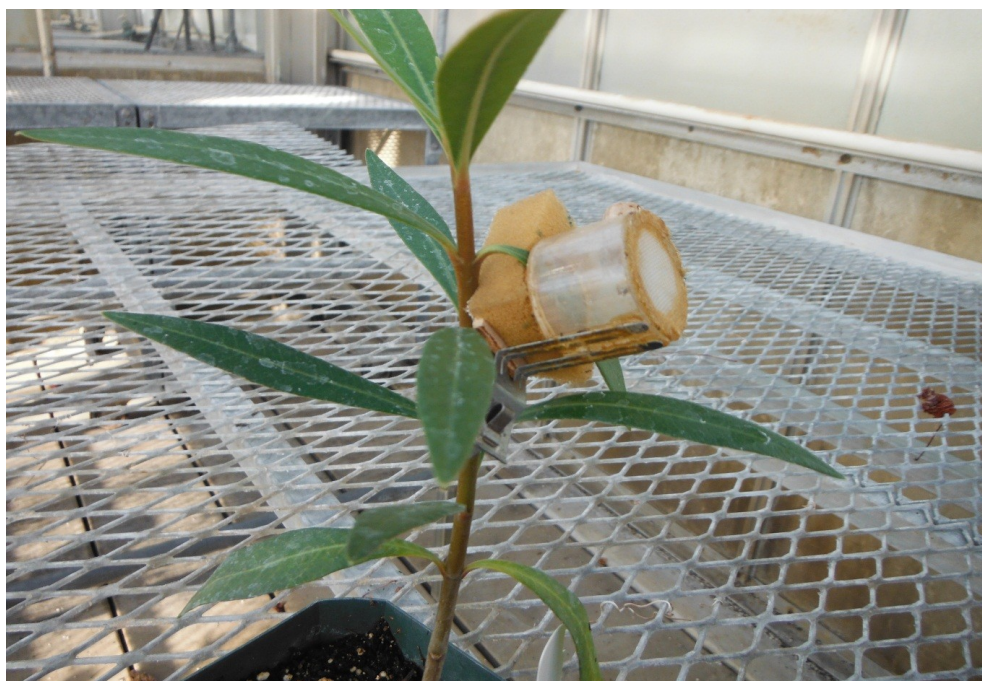
Figure 9. A small clip cage can confine vectors to a small area (2 cm). The cage glued to a hair pin and rests on foam rubber glued to one side of the pin. The cage has fabric on both sides but allows insects in the cage to feed through the mesh.
