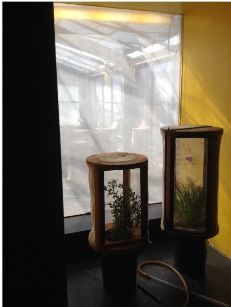
Figure 7. Bench for changing insect colonies or adding or removing insects from test plants in transmission experiments. Sunlight in the window and fluorescent light (top) attract the insects. The rear of the bench can be shielded with cloth to reduce insect escapes.
